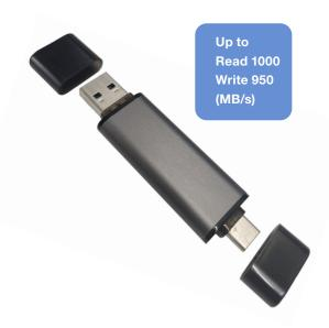
With 3D-NAND flash memory and a USB 3.2 Gen2 Type-A & C dual interface, the SuperTalent PS302 Portable SSD provides transfer speeds of up to 1000 MB/s, that's up to 4.9x faster than external HDDs. Transfers and backups of large-sized data including 4K videos and high-resolution photos will be much quicker and faster.
