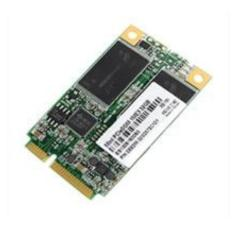
CORE STORE PLUS is a mini PCIe NVMe type Solid State Drive. It supports a max read speed of up to 130 MB/sec and a max write speed as fast as 100 MB/sec for Audio/Video Cache application. It also has a great performance of Random 4KB Read/Write up to 3.7K/9K IOPS.
