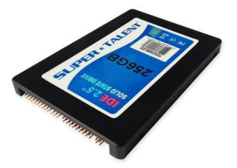
The DuraDrive ET is a solid state drive that provides high reliability and performance for industrial applications. The ET has excellent resistance to shock, vibration, dust, temperature extremes and other environmental hazards. It is built with the standard 2.5-inch form factor and a IDE(PATA) interface. This drive is geared specifically for the replacement of old IDE/PATA hard disk drives to improve the performance and reliability of old equipment.
