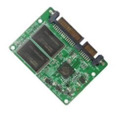
The SATA Slim SJ2 is one of many solutions for embedded and industrial system solid state storage. Systems that require a smaller form factor SSD can take advantage of the SATA Slim SJ2 transfer speeds for important applications that require read speeds up to 530 MB/s and write speeds up to 210 MB/s.
