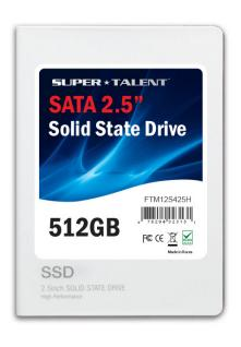
The SuperNova III features thermal conductive silicon padding and supports S.M.A.R.T. command. The reliability and speed of this SSD make it excellent for use in enterprise server workstations and for supercomputing. The SuperNova III helps to reduce TCO as well.
