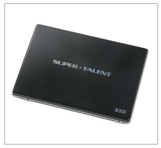
The MasterDrive IX2 is an industry standard 2.5-inch SSD with a parallel ATA interface. The MasterDrive IX2 more than doubles the performance of previous generations of IDE/PATA SSDs. Featuring Read Speeds up to 80MB/sec and Write Speeds 60MB/sec.
